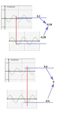
The resulting summing wave may look like in the following picture (just an example). And patching a quantizer between the LFOs and the VCO we get the following melody (given that we have chosen the output strenght of the LFOs adequately (later more about adequate modulation strengths).
