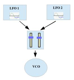
And we can – of course – adjust the LFO output strength differently for both LFOs.
