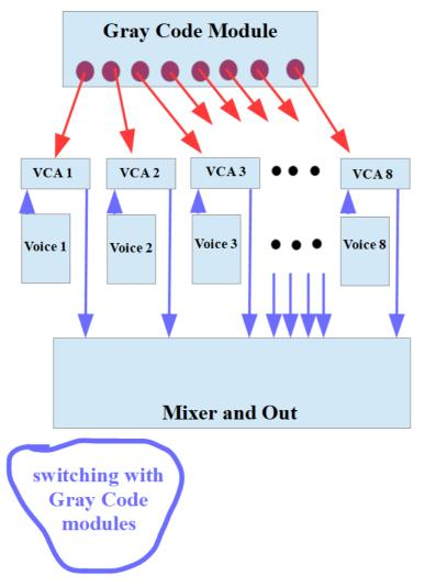
But a far more interesting way to switch between and merge whole voices (audio paths) is using ADSRs together with the VCAs, and patching the LFOs or the outputs of the Gray Code module(s) into the gain inputs of the ADSRs.
