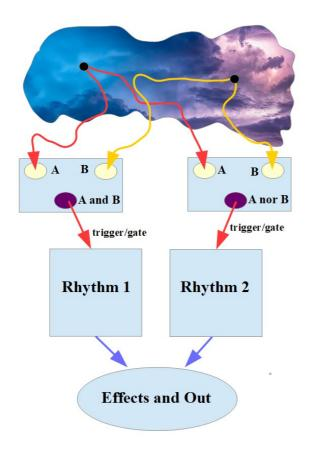
But we can use logic modules to really combine and expand rhythms as well. We can e.g. want an additional voice (bass, brass, whatever) to step in, always when the kick and the snare play together. Or we can want the additional voice (or another one) to step in only when neither kick nor snare are playing, or when only one of them is playing etc. The preset "voiceAdd.vcv" and the video behind the following link show this. https://youtu.be/iLiCDdhM6Mw
