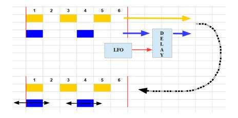
Another way to set up polyrhythms is using two sequencers with different numbers of steps per sequence an merge them, fade them in and out or switch between them to and fro. To introduce randomness I can use the obvious candidates (Bernoulli Gate, Gray Code module etc.) to do the switching and blending.
